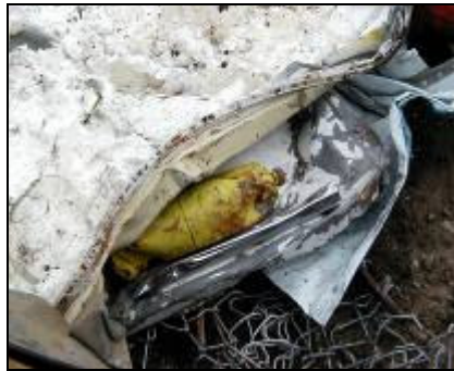
Prohibited: propane bottle inside a bale
