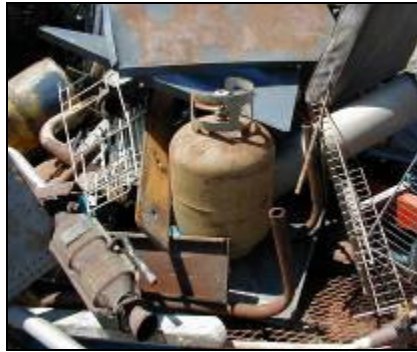
Prohibited: Propane tank commingled with other scrap
