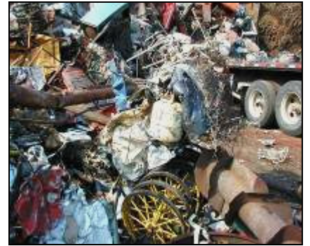
Prohibited: Propane tank commingled with other scrap
