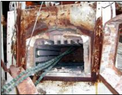
Prohibited: Kiln with radioactive refractory bricks
