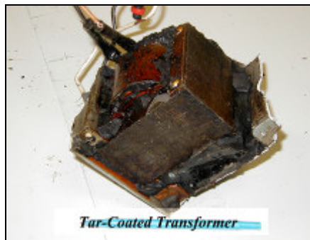
Prohibited: Tar-coated transformer
