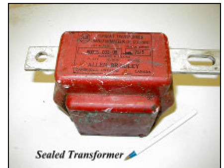
Prohibited: Sealed transformer
