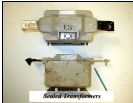
Prohibited: Sealed transformers
