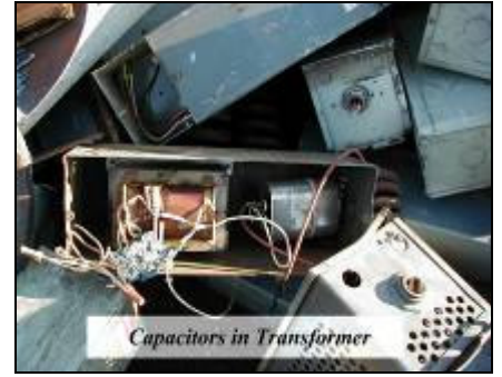
Prohibited: Capacitors in transformer
