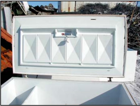
Mercury switch in a freezer
