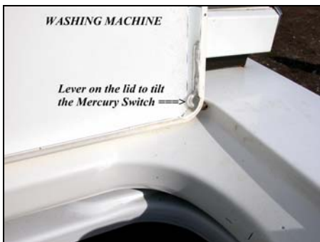
Washing machine with mercury switch
