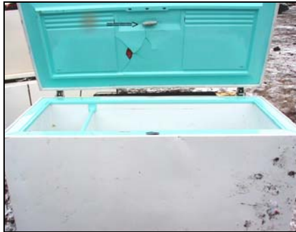
Mercury switch in a freezer
