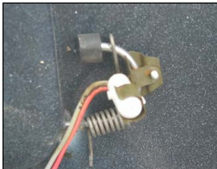
Mercury switch in a washing machine
