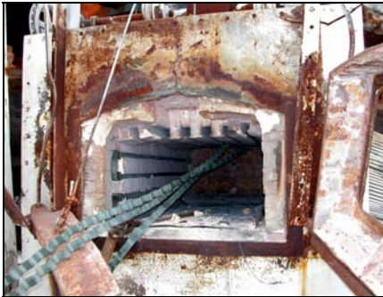
Prohibited: Kiln with radioactive refractory bricks
