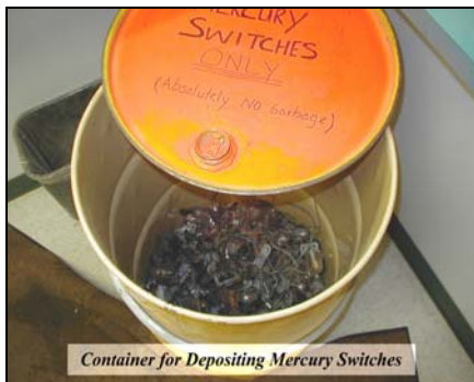
Container for holding mercury switches recovered by scrap recyclers
