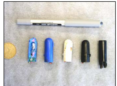
Mercury switches from washing machines
