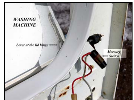
Mercury switch in a washing machine
