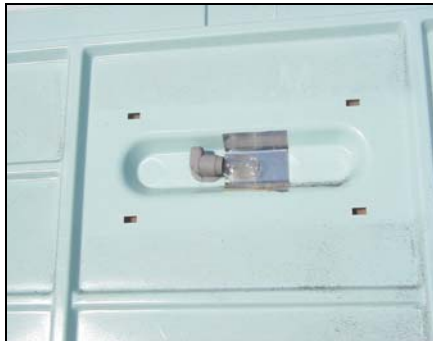
Mercury switch in a freezer
