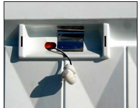
Removing mercury switch in a freezer
