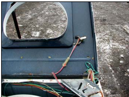
Mercury switch in a washing machine
