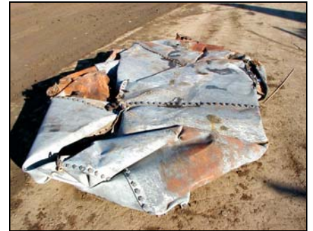
Prohibited: Storage tank with radioactive deposit / sludge
