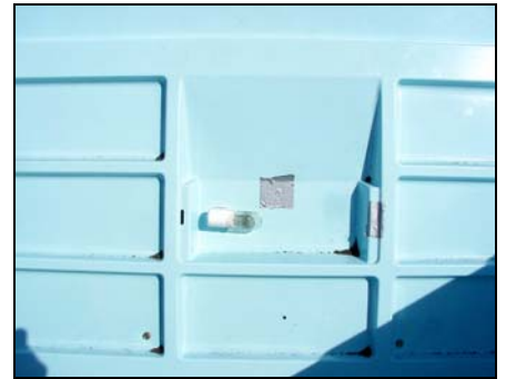
Mercury switch in a freezer
