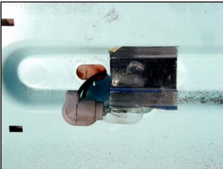
Mercury switch in a freezer
